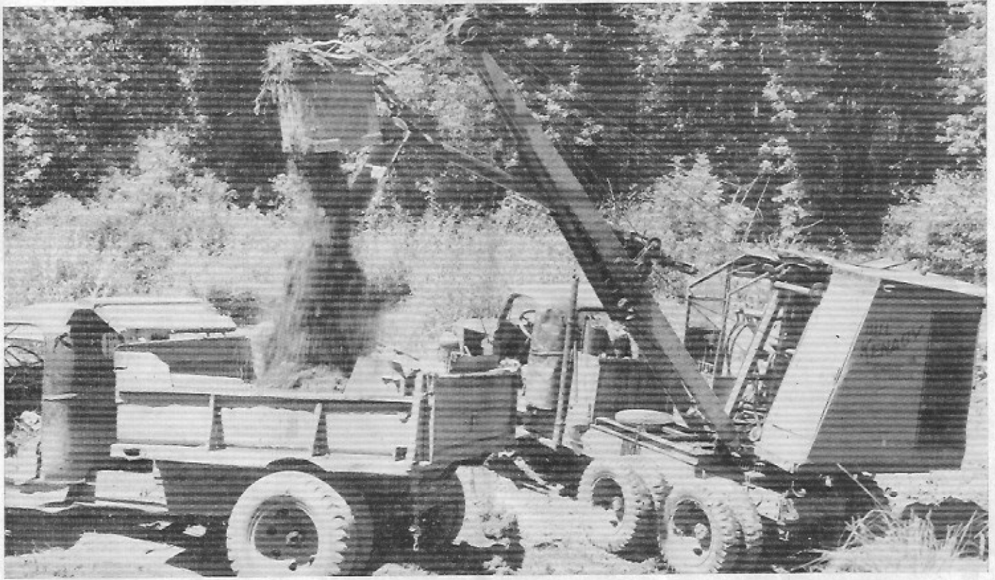
Clay is loaded by power shovel on a truck that will take it to the Needy Brick and Tile Factory of the Hubbard community. Frank Lais is operating the shovel.
